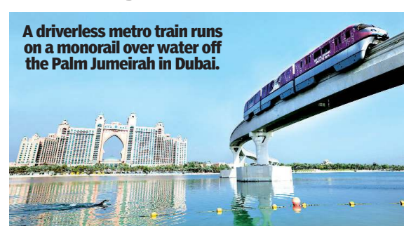
A driverless metro train runs on a monorail over water off the Palm Jumeirah in Dubai.
