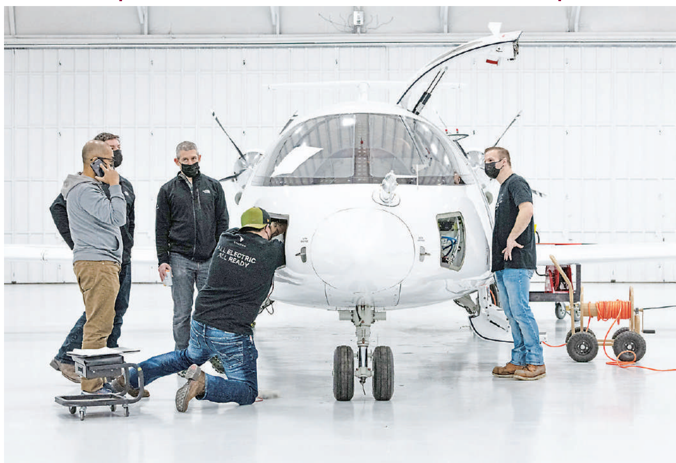
Aircraft engineers prepare Eviation Alice experimental electric aircraft for a taxi test in Arlington, Washington, US.
